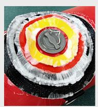
done in the photo at left is fit 6 different polyure-thane material samples under the valve, removed the O-ring seal, and inflated to standard operating pressure. This allows air to travel up the valve nut threads and access the valve hole at centre of each of the sample discs. The detergent solution
